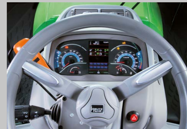
The new InfoCentre provides an overview of operating conditions – in both digital and analogue mode.
