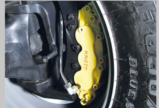
Wet disc brakes on the front axles for extra-safe braking effect (optional).
