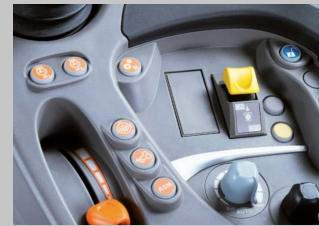
The PTO settings and activation are conveniently integrated into the armrest ...
