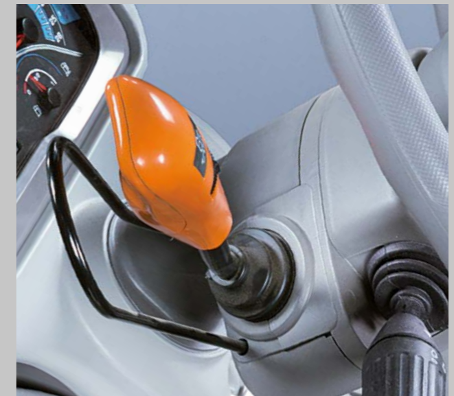
Standard: Hydraulic power shuttle system. The shuttle sensitivity (hard – medium – soft) can be easily adjusted with the thumb.
