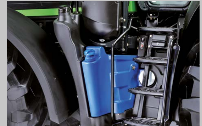
600 l diesel and 55 l AdBlue are sufficient for more than one day of hard work in the field. Optional: Fuel pre-filter for the best cold-start performance.
