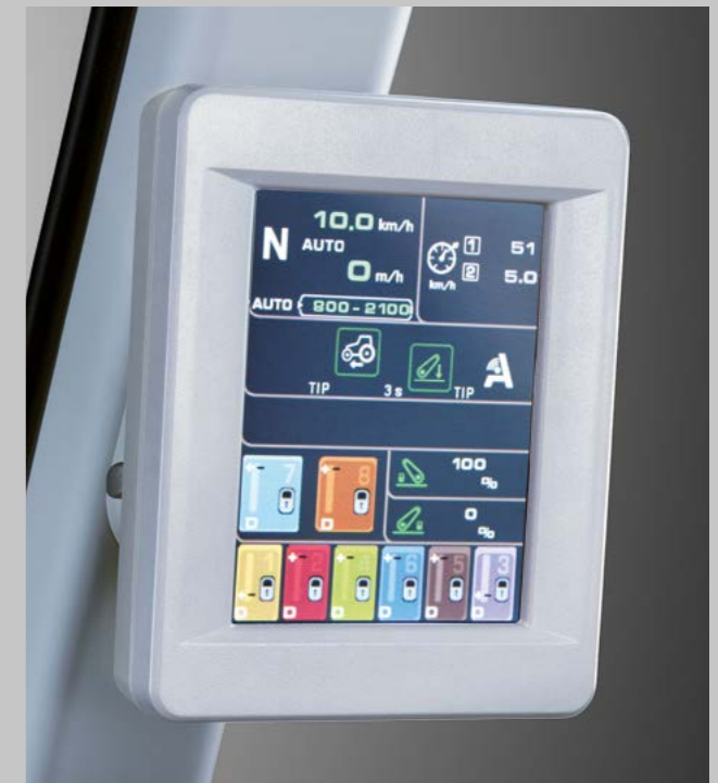
Three driving or work strategies can be selected. Manual, automatic and PTO. They are displayed in the WorkMonitor.
