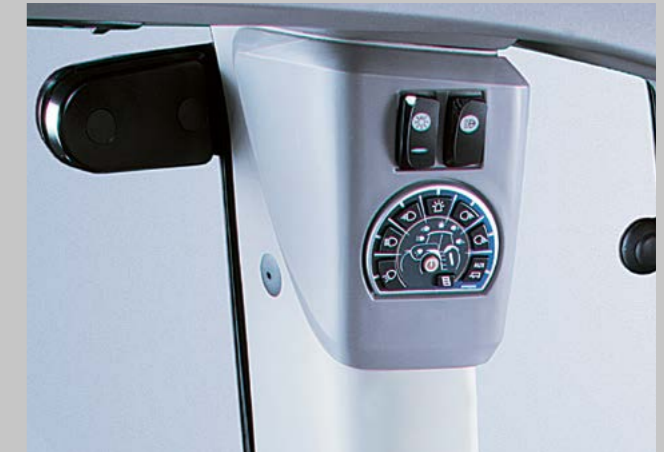
Driving lights, work lights and cab light combined in a single control panel.
