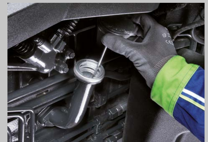
Checking the oil level and topping it up is also incredibly simple.
