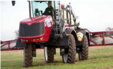
Crab steering - in difficult conditions and manoeuvring
