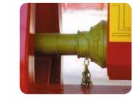
1,000 to 540 gear, it is possible to use tractors that cannot operate at both PTO speeds
