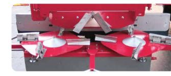
For spreading compost, sand and heavy materials, the direction of rotation (off centre) off the spreader discs can be changed. This feature is available in two ways on the SPC4500-1 and 2 spreading boxes.
