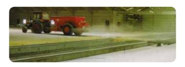
BREDAL spreaders work according to the double-overlap principle, i.e. at a spreading width of 12 m, the actual spread is 24 m. This principle ensures correct spreading.
