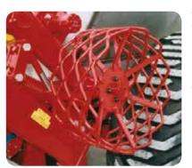
The mechanical drive wheel transfers the vehicle's speed, enabling the application rate to be adjusted according to the forward speed. The drive wheel is simply and robustly built and can be adjusted to suit different treads and wheel sizes. The drive wheel has a spring pressure of 400 kg. This guarantees that the vehicle wheel peed is always transferred accurately to the nveyor belt.
