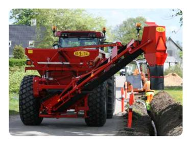
Bredal sand spreader. For mounting on type K45-K105.
