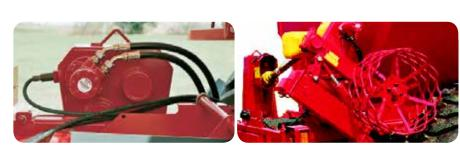
For electrical/hydraulic operation, the belt is controlled via a valve and oil motor. This facilitates spreading of large or small amounts. If required, the spreading wheel can remain in the machine as a backup, for example, if it becomes necessary to use a tractor that does not have a computer installed.
