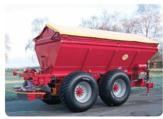
K135 with 650/65 x 30.5 tyres, 12-16 m lime/12-24 m fertilizer equipment and hopper extension with hydr. cover. K135 comes as standard with hydr. dosing control via Bredal LH500 computer.
