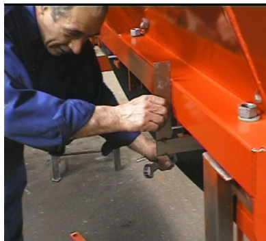
14. Adjust the distance from the external frame in to the belt roller frame to obtain a centred position.
