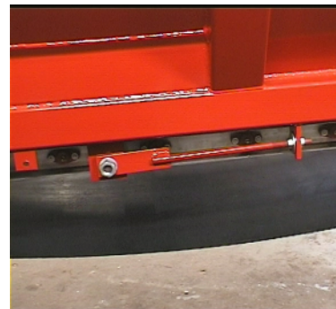
15. Adjust the belt frame so the belt roller runs vertically on the belt roller beds (see fig. 16).
