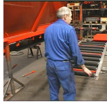
9. Push the belt roller into the conveyor belt (be extremely careful - the sharp edges can cut both the belt and your HAND!!).
