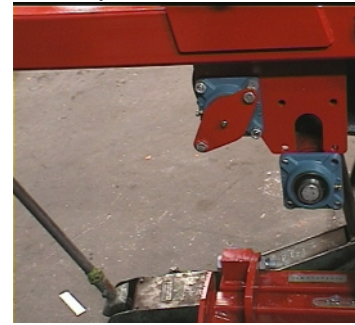
12. Lift the snap roller (the belt tightener at the back roller) up into place
