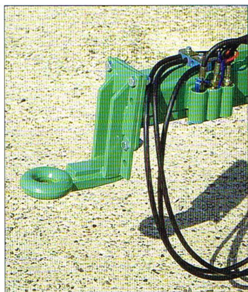
Supports des raccords hydrauliques.
