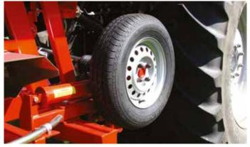
The hopper floorbelts are driven mechanically by a wheel pressed firmly against the tractor rear wheel, for constant application rate independent of forward speed. The drive wheel can be adjusted sideways and for length to match different tractors and track widths.
