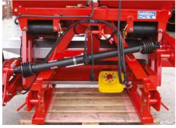
Frame construction strongly built for an accurate weighing and for many years of intensive use. The adjustable drive wheel can be adjusted to different track widths and wheel sizes of the tractor.
