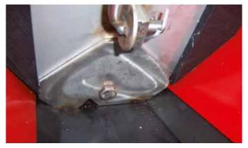
A reduction Kit can easily be fitted without tools for application of small seeds or slug pellets.
