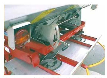
As an option on the F2WS and F2S, the downshutes can be automatically adjusted as the amount of fertiliser coming onto the disc varies with the forward speed. Experience and extensive tests have confirmed the importance of the dynamic placement of the fertiliser on the spread discs in order to obtain the best possible distribution of the fertiliser.
