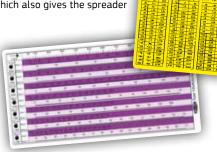
BREDAL spreaders work according to the double-overlap principle, i.e. at a spreading width of 12 m, the actual spread is 24 m. This principle ensures correct spreading.
