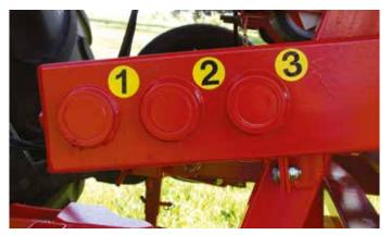
Drive to the floorbelts with 3 speeds for low to very high rates, is through a heavy duty gearbox. This positive, equal feed ensures precise control of the application rate, which is unaffected by different fertilisers or weather conditions.
