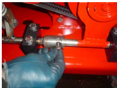
10) Handle to be moved in middle position and mount lock pin..
