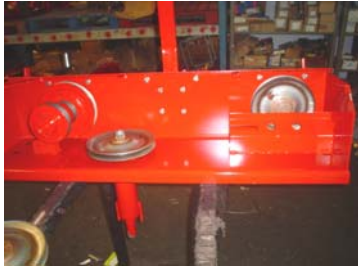
1) Spreadbox without V belts
