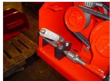
9) Feder guidance and feder to be mounted
