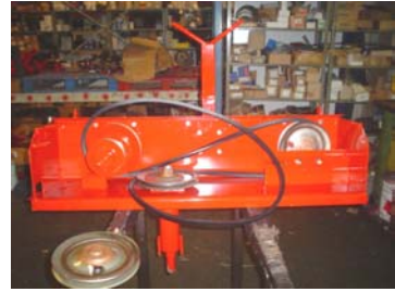
3) twist 180° and around pulley on headland gear
