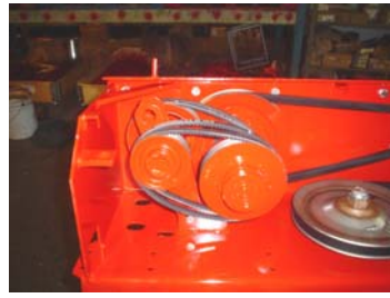
5) Tightening on headland gear to be mounted with V-belts.
