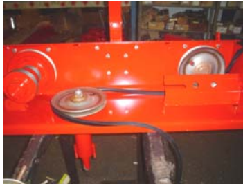
2) V-belt around pulley 1 and 2
