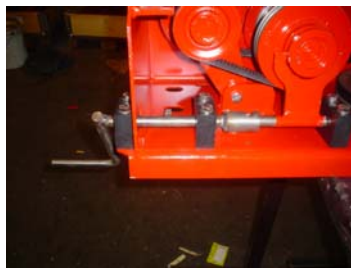
8) Handle and plastbearing 2 and 3 to be mounted
