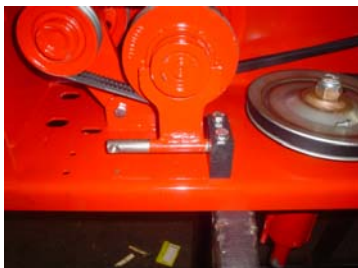
7) Changing fork and plast bearing 1 to be mounted
