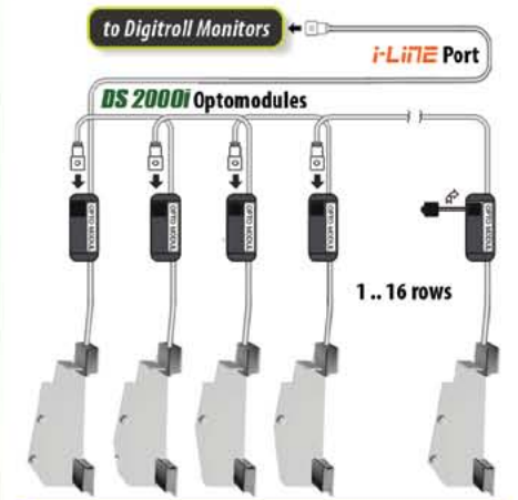
APPLICATION EXAMPLE WITH DS 2000i: • i-LiNE Port: 16 rows precision planter control
